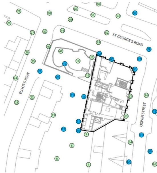
Image 44 (above): Wind effects map of the proposed development with existing surrounding buildings and existing landscaping in the windiest season.
