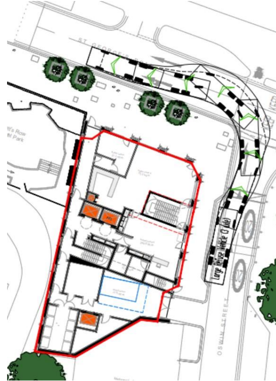
Image 40 (above): Tracking diagram of the left-turn manoeuvre from Oswin Street into St George's Road.
